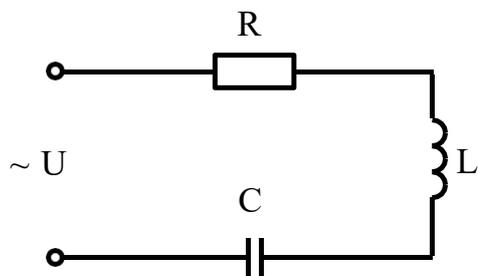
1)  $Z = \sqrt{R^2 + \left(\frac{1}{\omega L} + \omega C\right)^2}$ ; 2)  $Z = \sqrt{R^2 + \left(\frac{1}{\omega L} - \omega C\right)^2}$ ;
